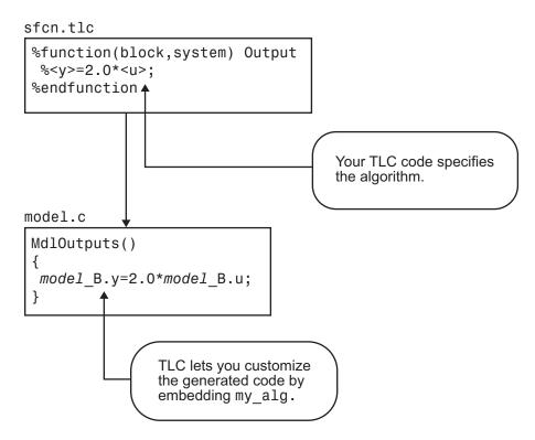
The S-function timestwo.c provides a simple example of a fully inlined S-function. This block multiplies its input by 2 and outputs it. The C MEX version of the block is in matlabroot/toolbox/simulink/simdemos/simfeatures/src/timestwo.c, and the inlining TLC file for the block is in  $matlabroot/toolbox/simulink/simdemos/simfeatures/tlc_c/timestwo.tlc.$
