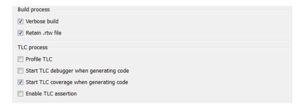
When you initiate TLC coverage, the Target Language Compiler produces a .log file for every target file (\*.tlc) used. These .log files are placed in project folder created for the model. Each .log file contains usage (count) information regarding how many times it encounters each line during execution. Each line begins with the number of times it is encountered, followed by a colon, followed by the code.
