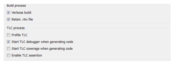
Selecting **Start TLC debugger when generating code** is equivalent to specifying the TLC option -dc on the **Code Generation** pane of the Configuration Parameters dialog box.
