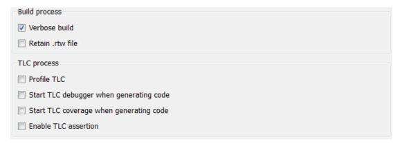
The **Start TLC debugger when generating code** check box lets you activate the TLC debugger. This is covered in more detail in "Debugging".
